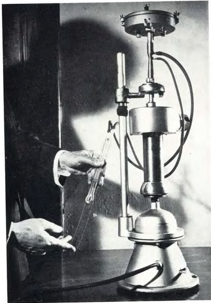
FIGURE A 4. SIEVE ANALYZER IN TANDEM WITH AIR CENTRIFUGE. Operating 1/2 foot per minute it simulates aerodynamic constants of respiratory system; dust particles collect in "sieve" and droplet nuclei in centrifuge; the sieve corresponds to the upper respiratory passages and the centrifuge to the lung. See Chapter iv. Photograph by Larry Keighley. Reproduced by permission
