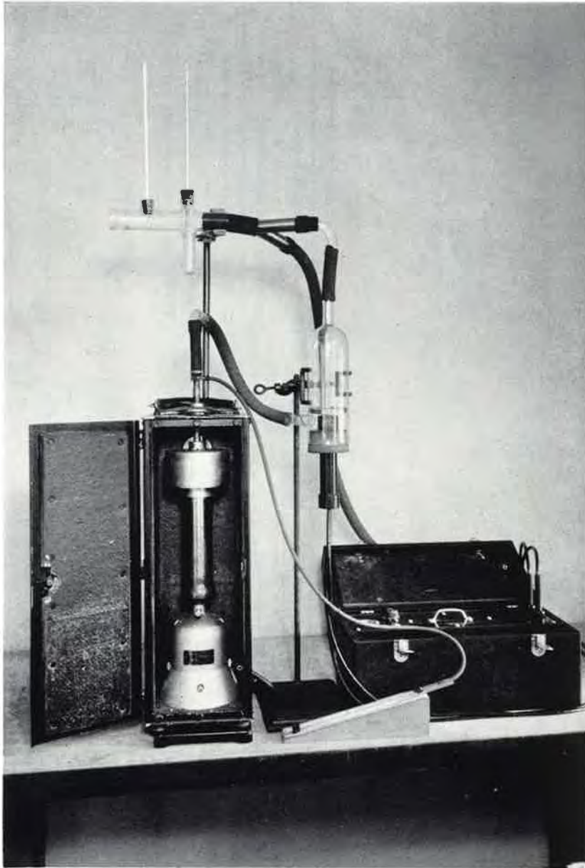
FIGURE A 18. STANDARDIZED IRRADIATION OF AIRBORNE MICROORGANISMS. Assembly for measuring vulnerability of organisms to ultraviolet light. See Chapter VII
