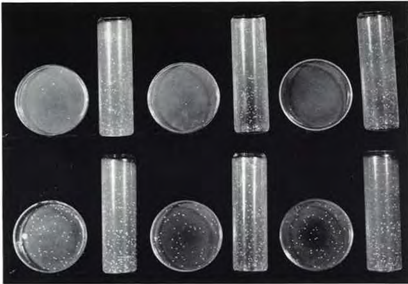
FIGURE A 22. TYPICAL TESTS OF SETTLING VELOCITY OF FINE (upper row) AND COARSE (lower row) AEROSOL SUSPENSIONS indicated by similar counts on centrifuge tubes but different counts on the settling plates. See Chapter x
