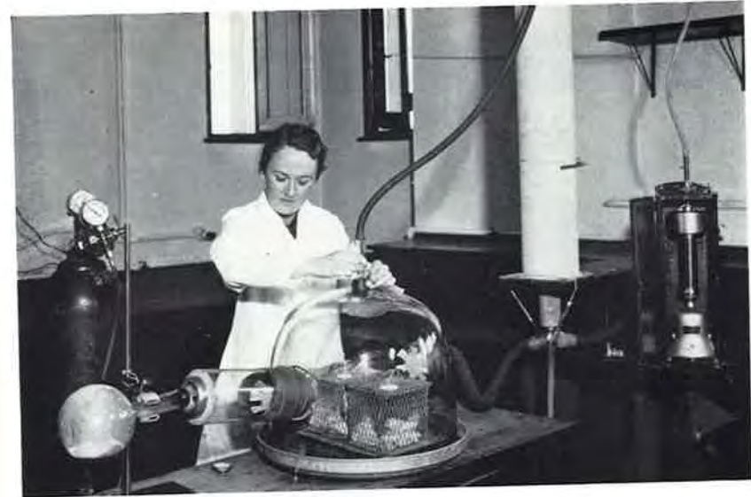
FIGURE 18. FIRST INHALATION CHAMBER. Wells apparatus for quantitative infection of animals by inhalation. See text
